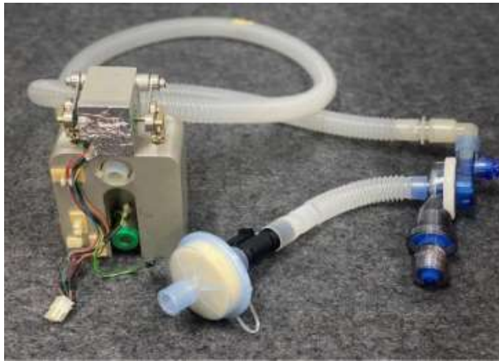
Figure 2. The two double-acting pistons pump system in experimental tests.
